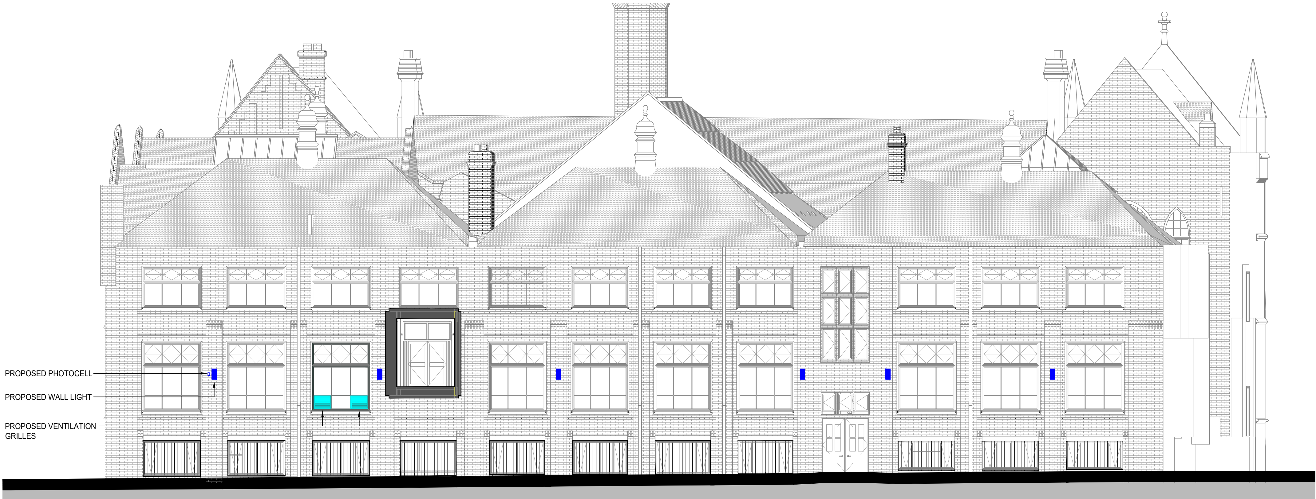
EXTERNAL LIGHTING ELEVATION (SCALE 1:100)
