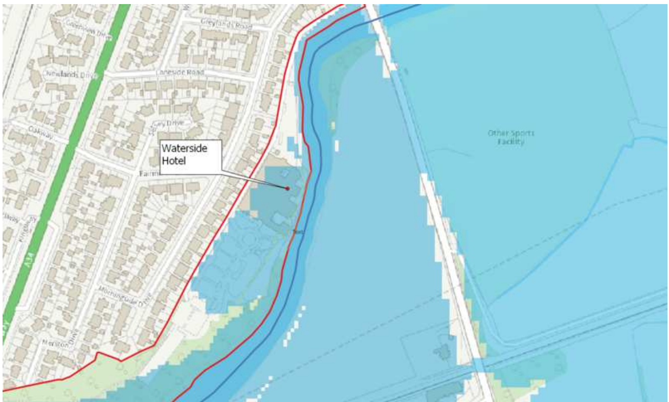
Figure 3.2: Hydraulic Modelling Results - 1 in 100 year flood levels
