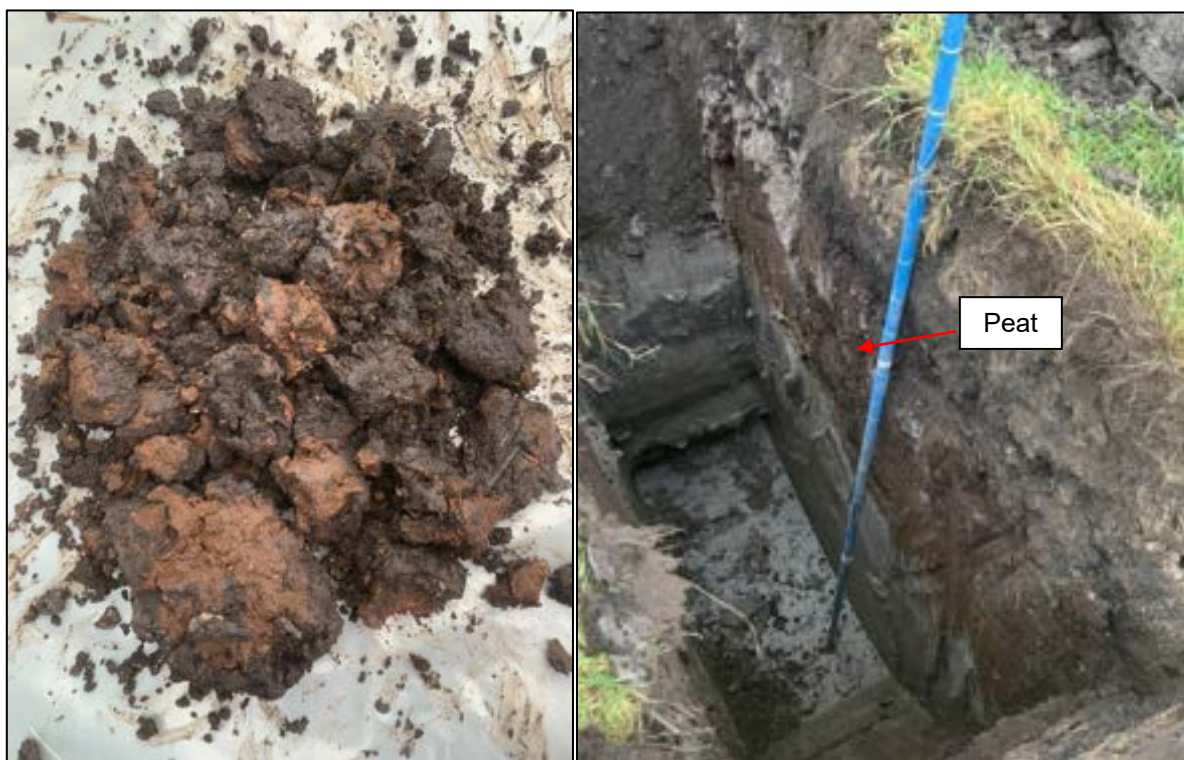
Figure 4: Photographs of the typical peat deposits encountered on site (left) and the peat in situ within TP10 (right).
