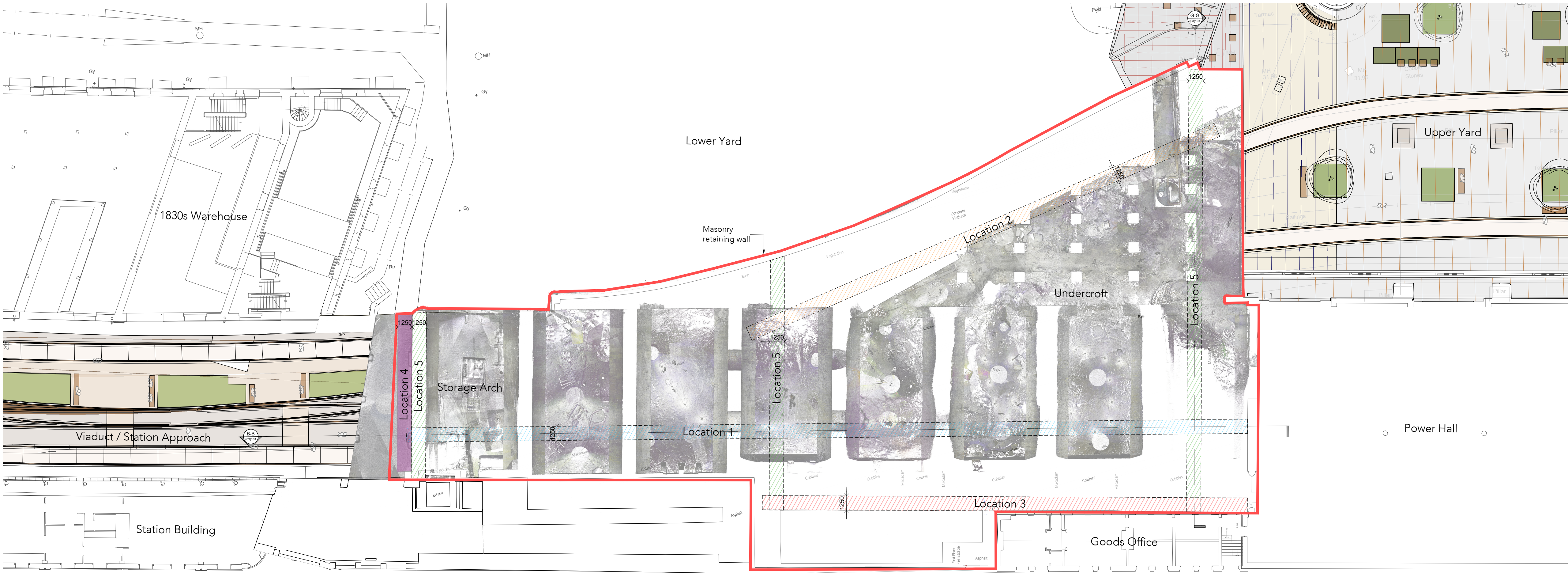
Goods Office Yard Lower Level Plan as Existing - Proposed Trench Locations Scale 1:200
