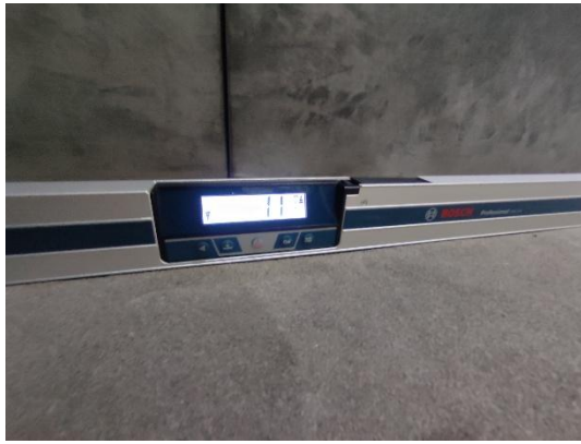
Photo 29 – Inclination of floor recorded as 11mm per meter in areas.
