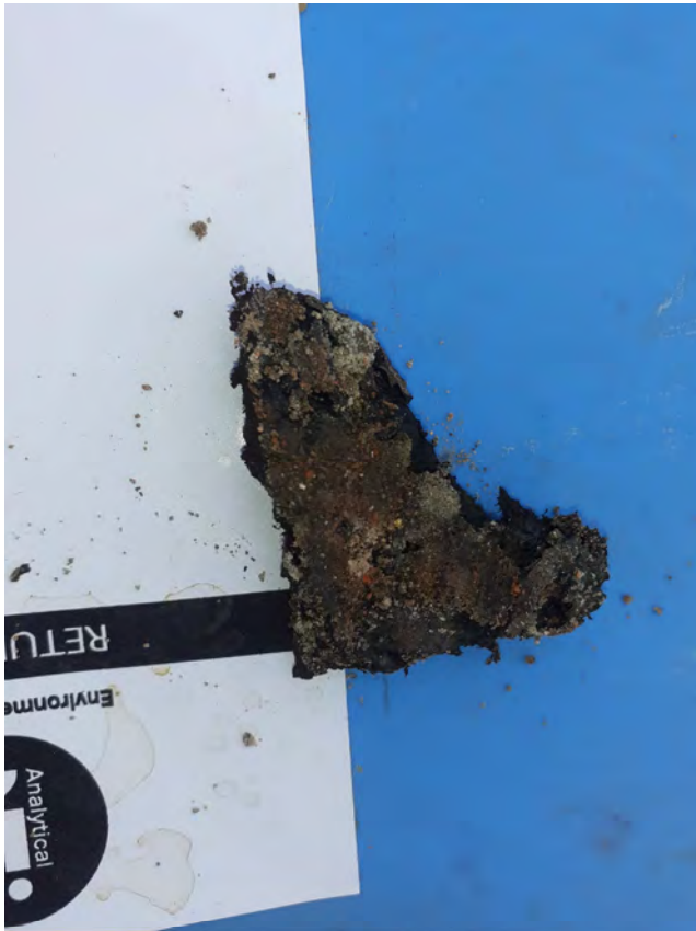
Bitumen Pipe (Chrysotile)
