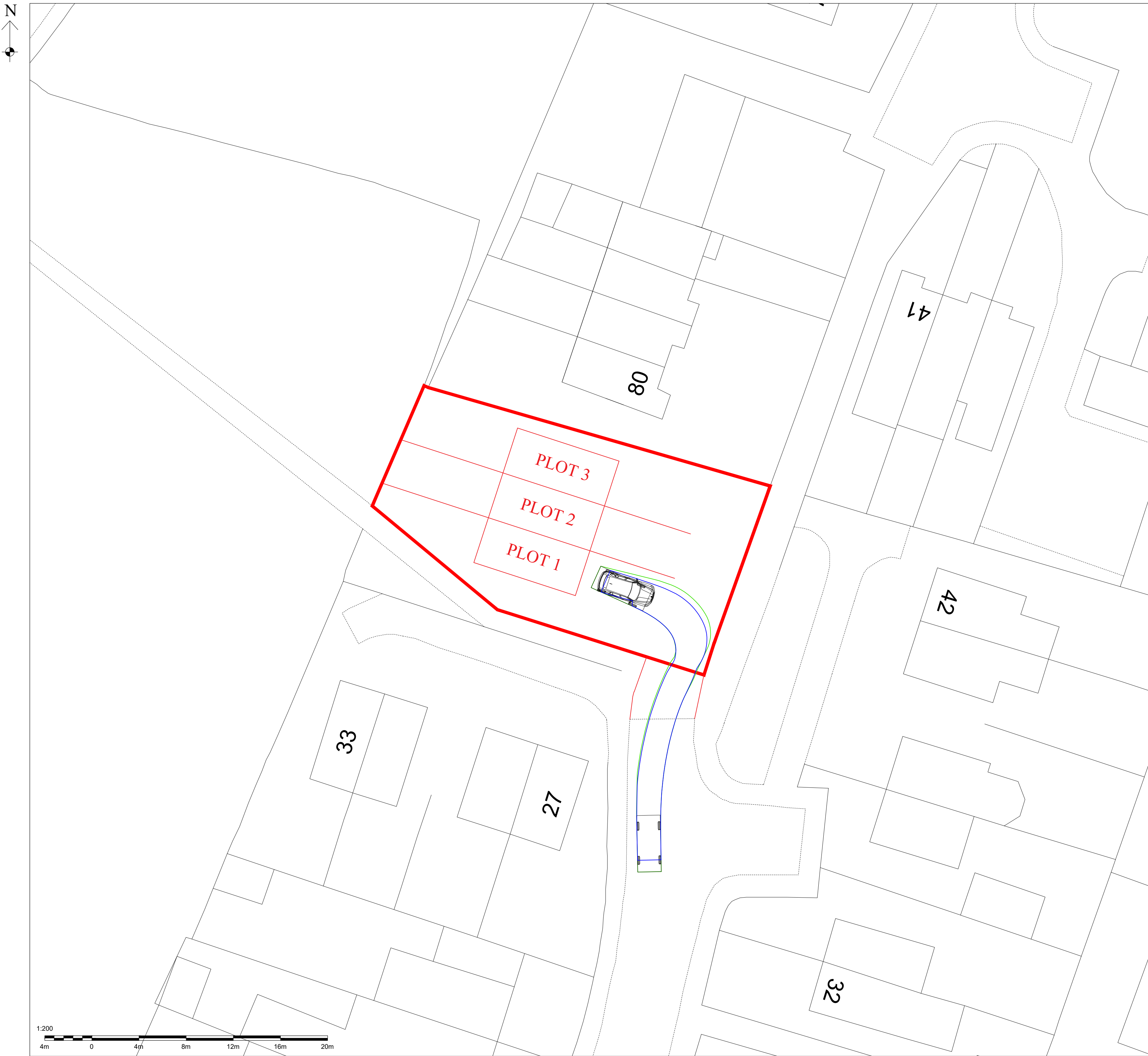
PLOT 1 PROPOSED VEHICLE ACCESS (SCALE 1:200)
