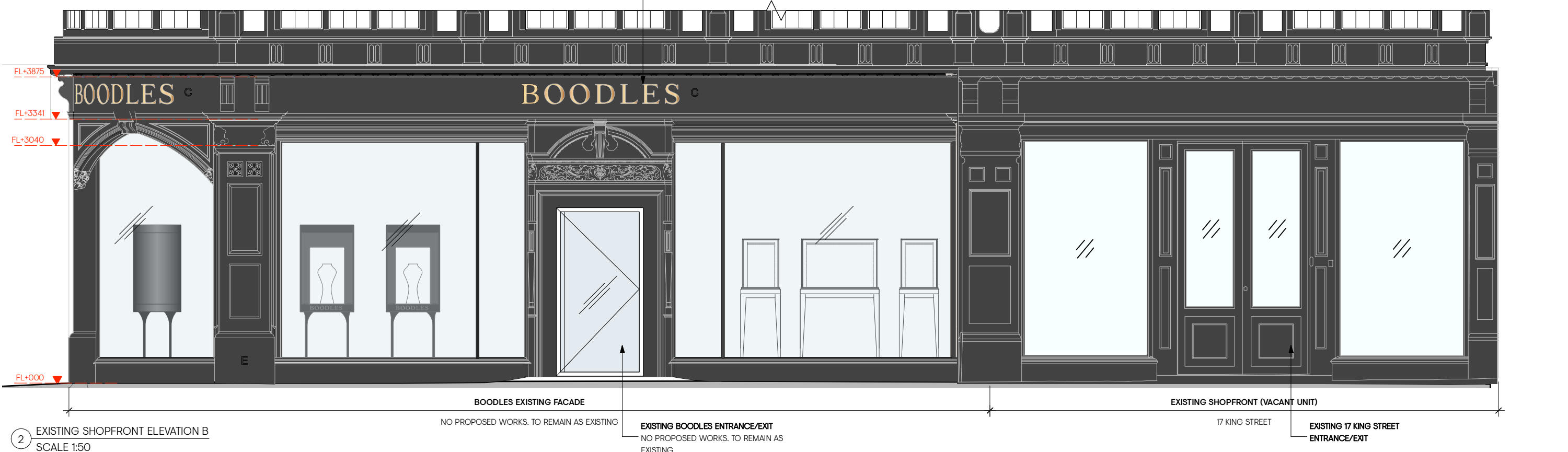
1 EXISTING SHOPFRONT ELEVATION A SCALE 1:50
