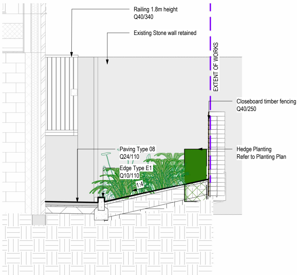
2 Elevation through north facade facing west 1: 50 @
