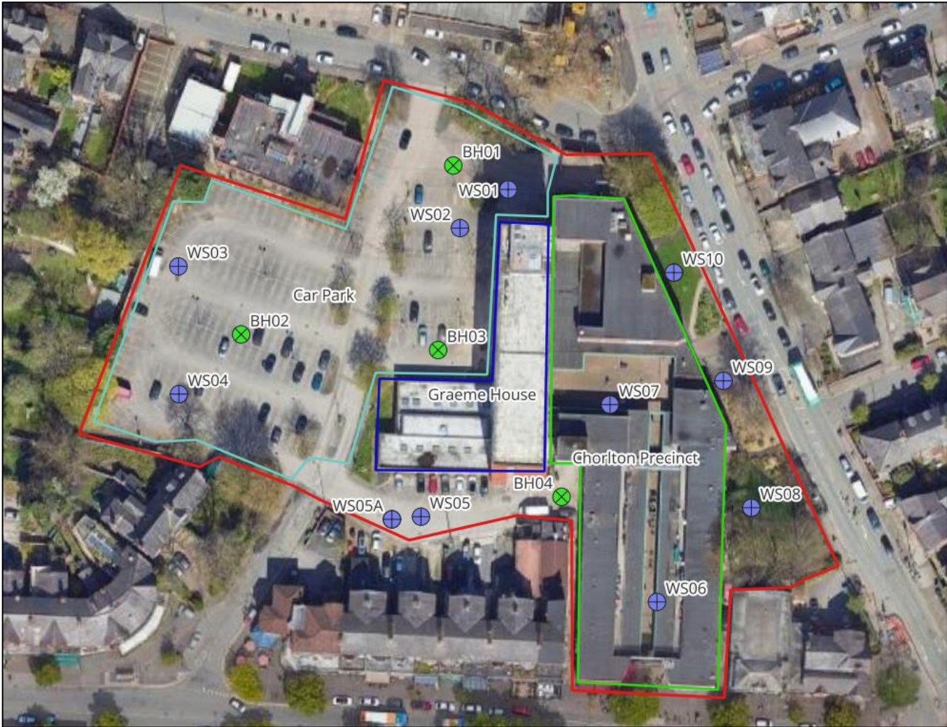
Figure 6: Borehole locations from Phase 2 site investigation
