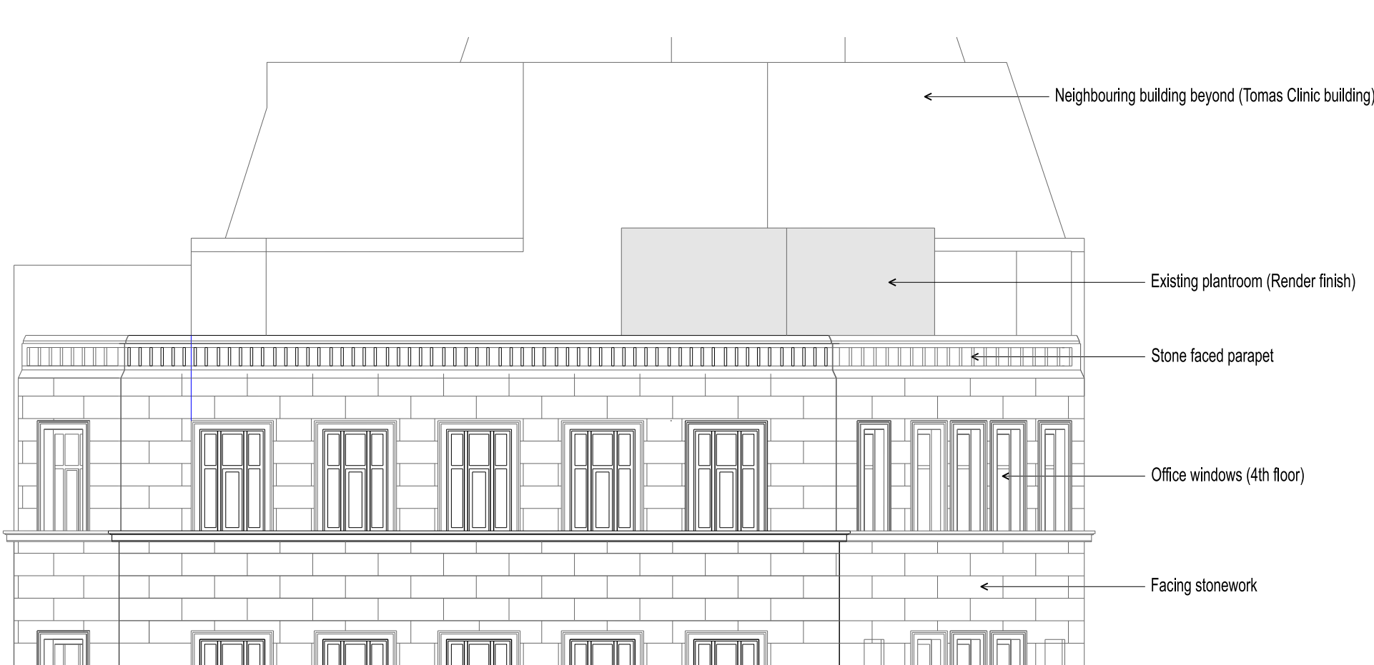
WATSON STREET ELEVATION - EXISTING 1:100
