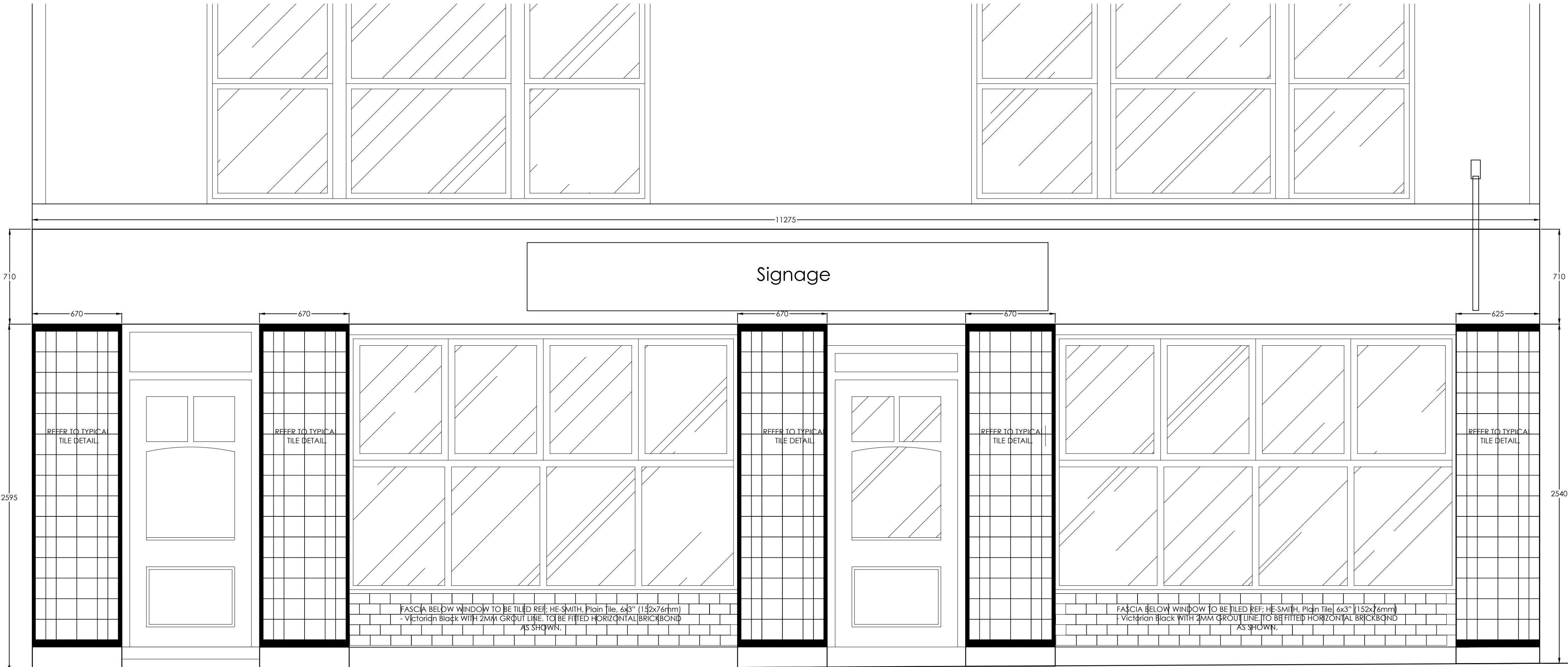
FRONT ELEVATION - TILING DETAIL 1:20
