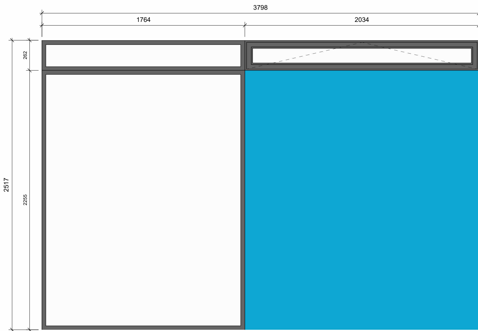
1 Existing Window Elevation Type A 1 : 20
