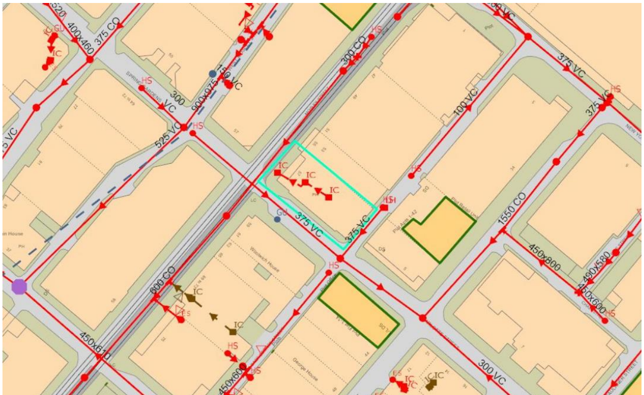
Figure 7.2: United Utilities sewer records
