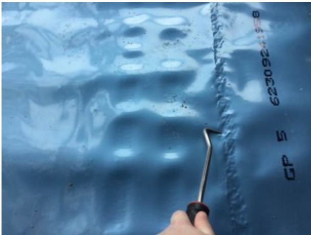
Pick testing along the hand welded lap joint.
