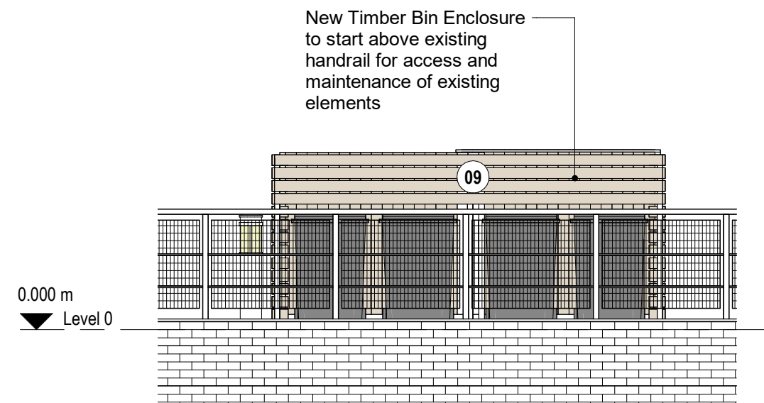
H Bin Enclosure - Elevation H 1 : 50 @ A1
