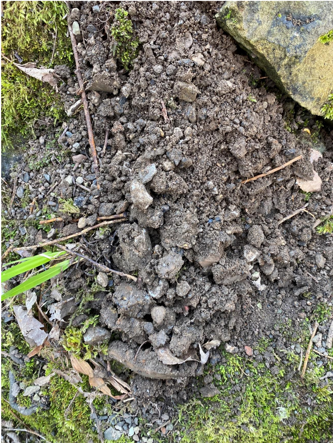
PLATE 1 HA105 ARISINGS TYPICAL OF THE EMBANKMENT
