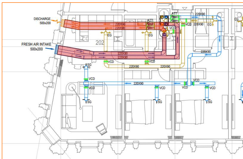
Figure 2: Typical Ventilation Layout
