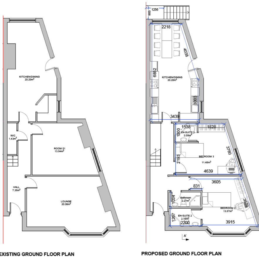
Figure 3. Existing and proposed ground floor plans (HAD & Co 2025)
