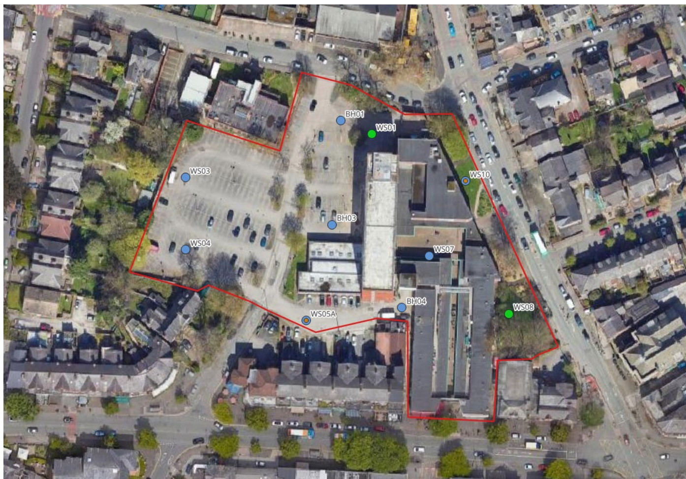
Plate 10: Summary of Made Ground Soil Contaminant Exceedances from Site Investigation
