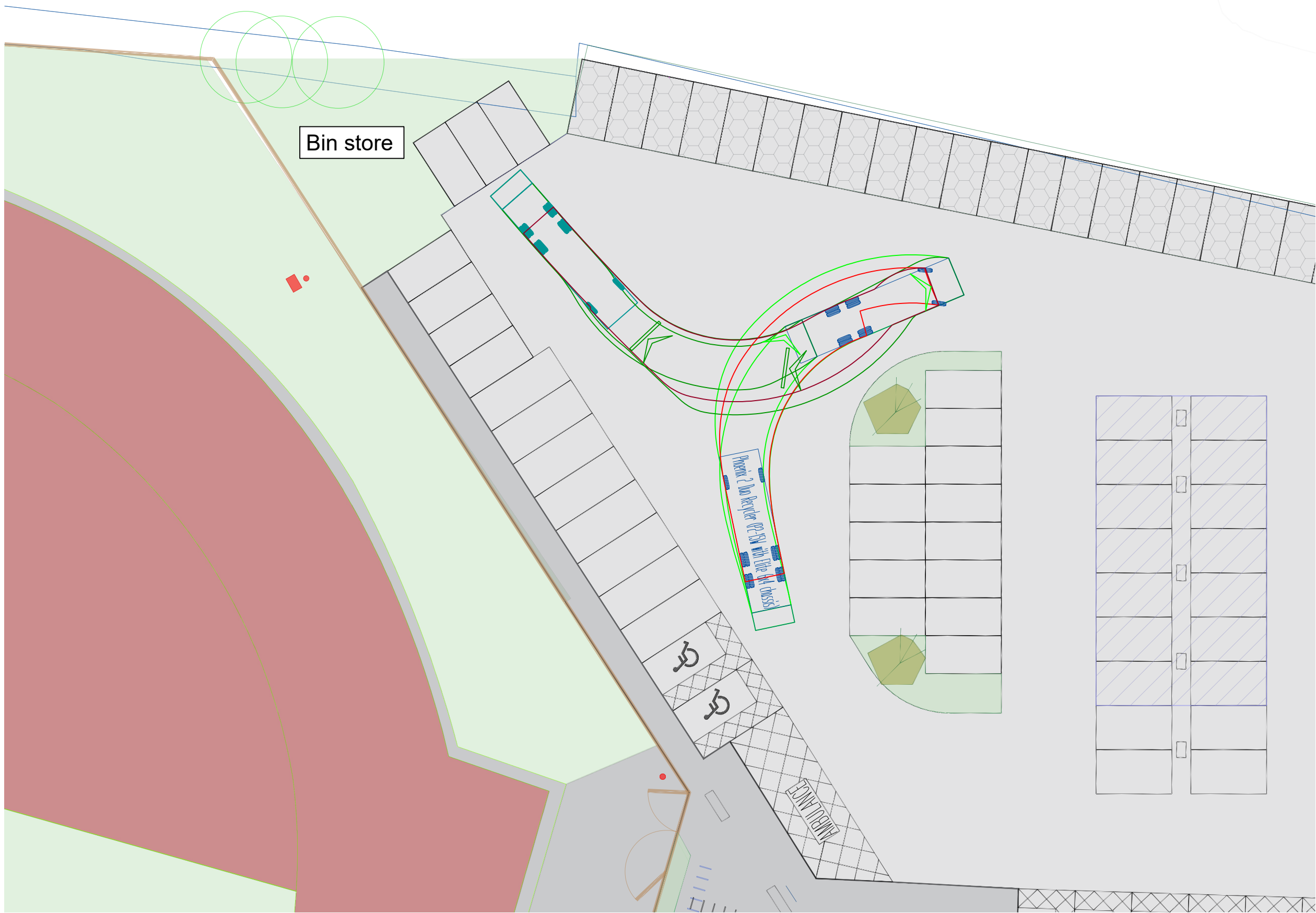
Swept Path - Reversing to Bin Store Reverse Speed - 2.5mph (Scale 1:250)
