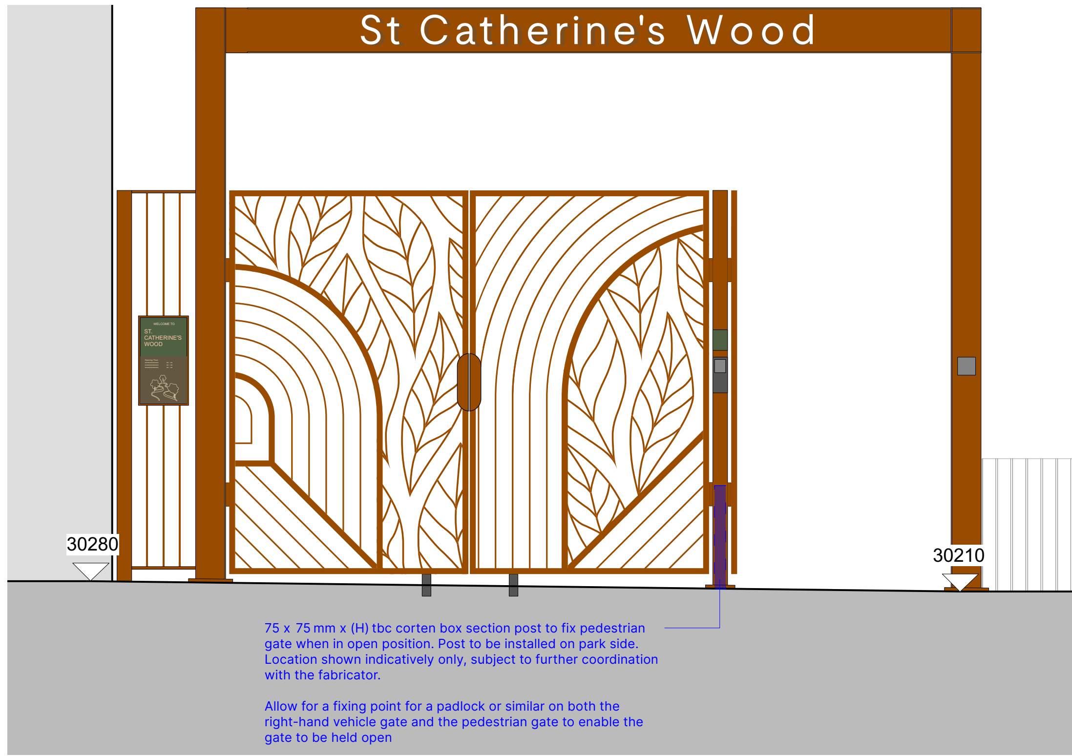
3 Gate & Fence Detail - pedestrian gate open Scale: 1:25
