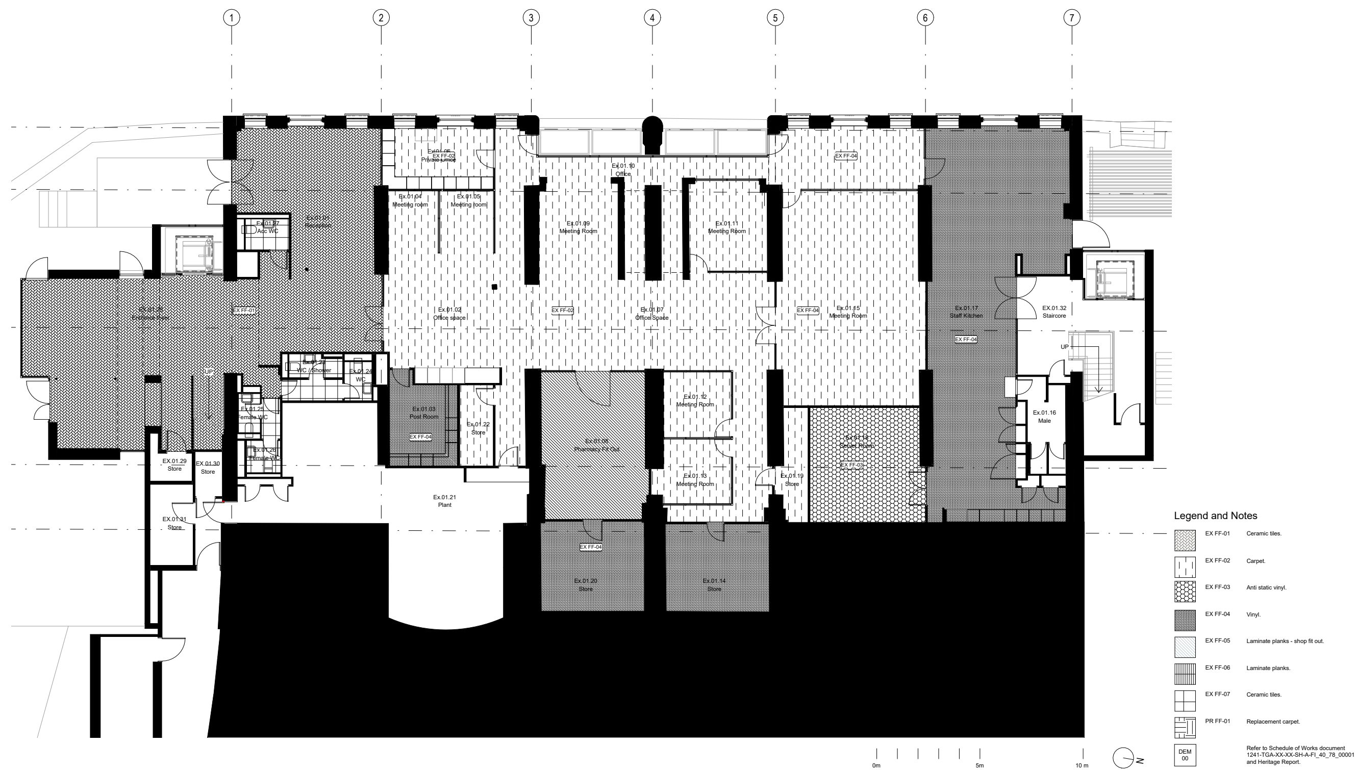
Level 01 - Existing Floor Finishes Plan
