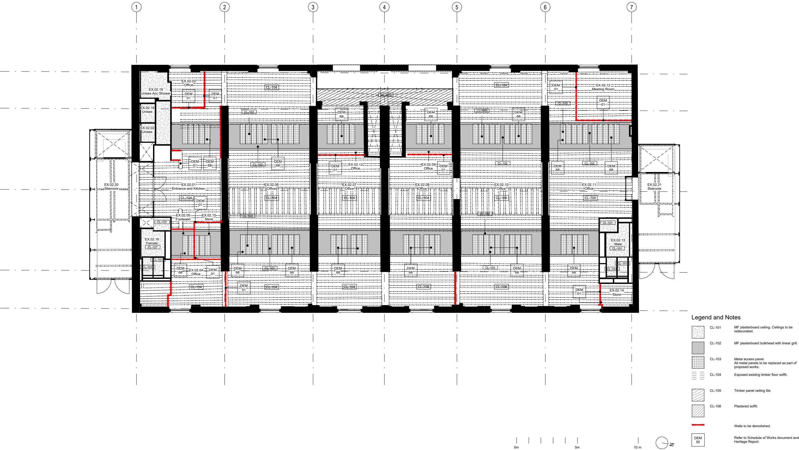
Level 02 - Demolition Ceiling Plan
