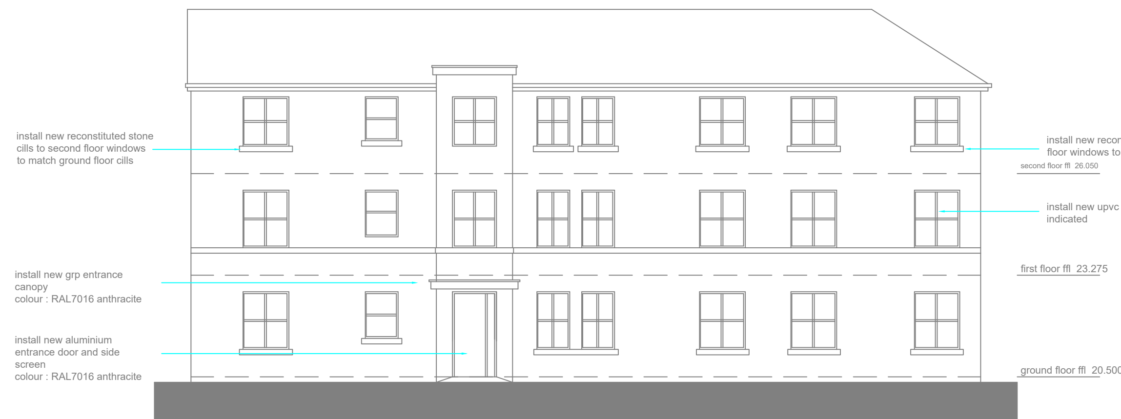
FRONT ELEVATION (elevation to rochdale road) (scale 1:100)
