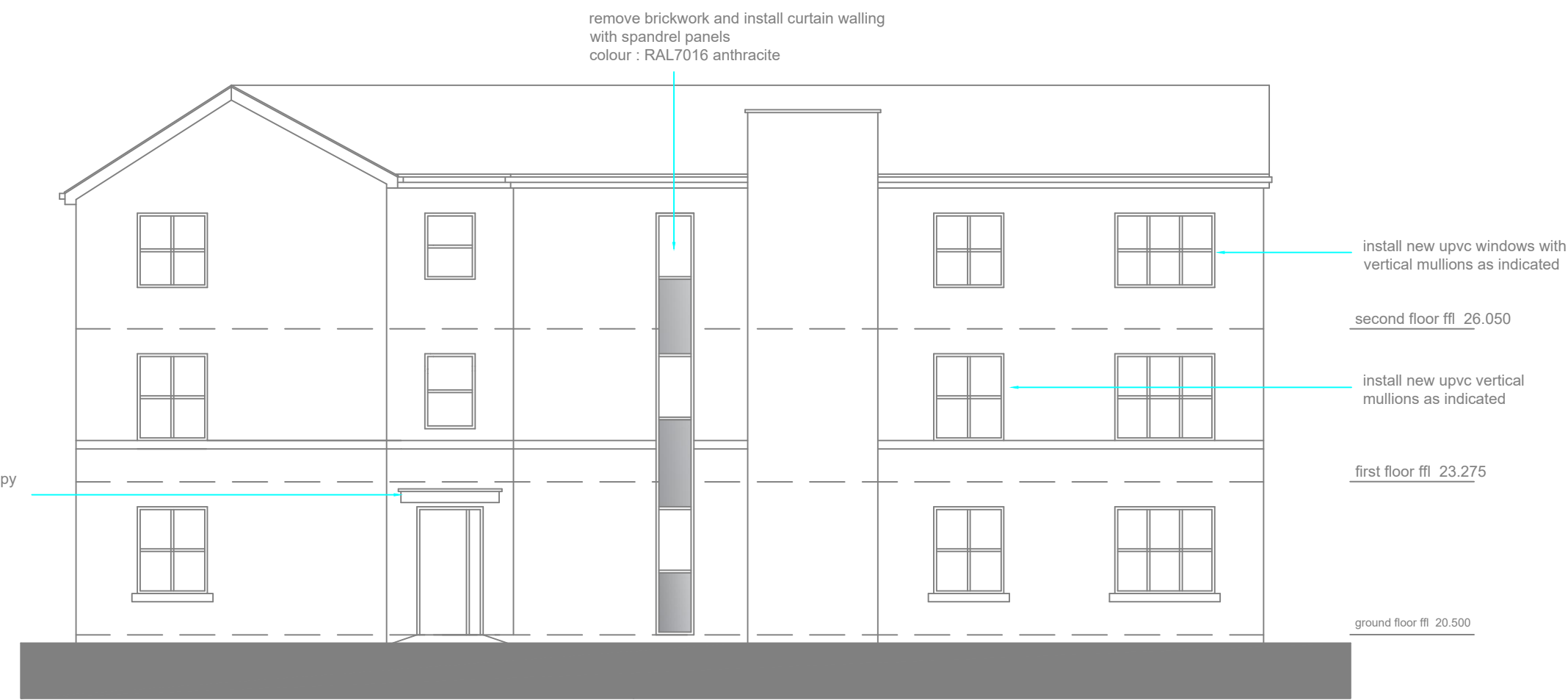
REAR ELEVATION (elevation to car park) (scale 1:100)
