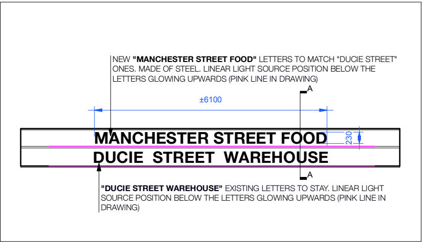
DETAIL ELEVATION OF PROPOSED SIGNAGE | SCALE 1/100 @ A3
