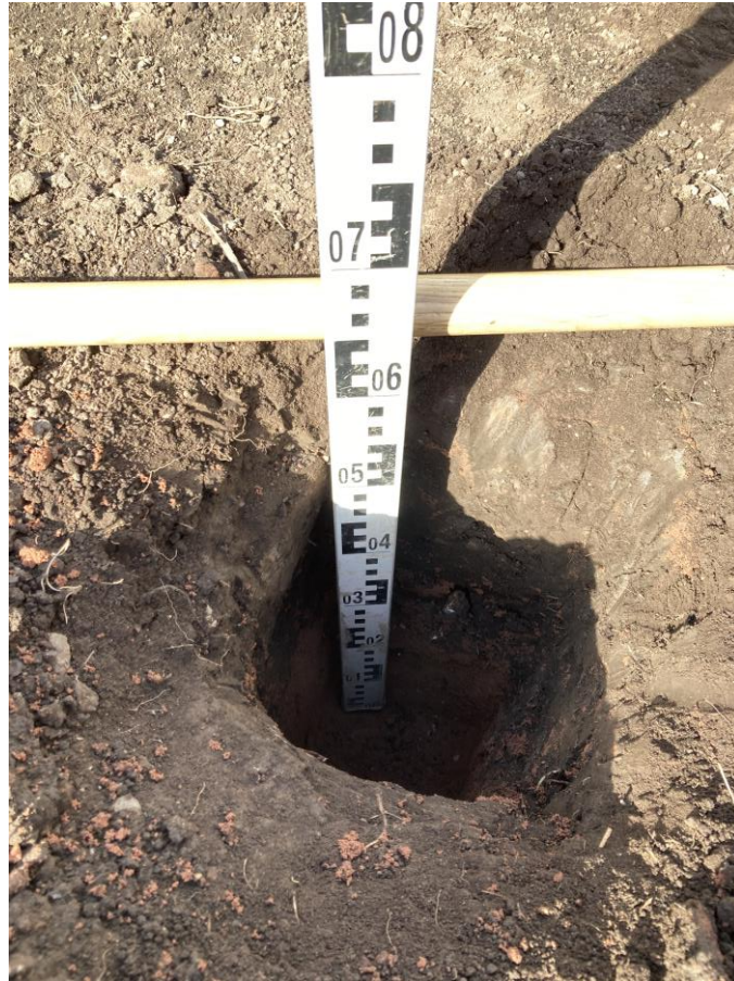
Photograph 10 250mm of topsoil and 400mm of subsoil emplaced in VP03.
