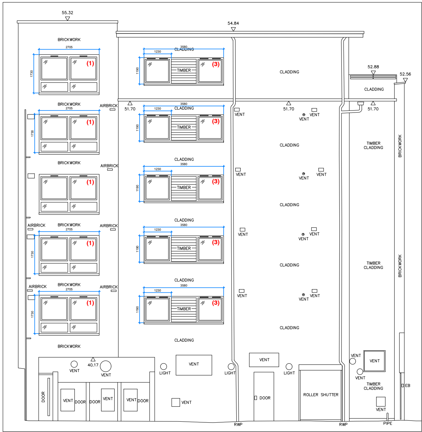
EXISTING ELEVATION REAR OF BLOCK SCALE 1:00@A1
