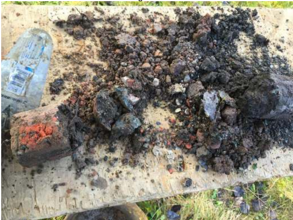
Photo showing the Made Ground found on site
