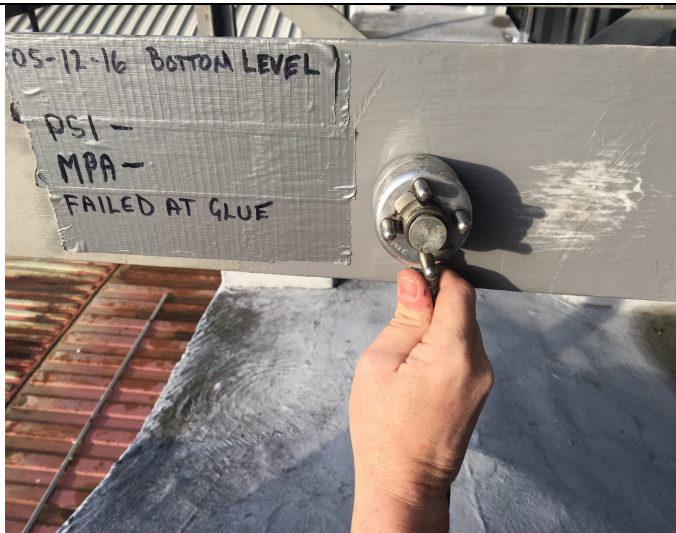
failed at glue (no result obtained)
