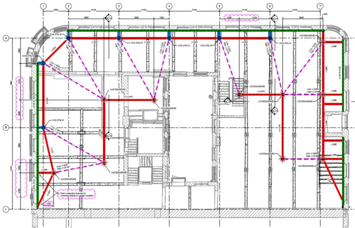
Figure 4 Plan Showing Typical Restraint Framing
