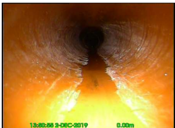
Photo: 24_2A 0m, Clear water level, 5% of the vertical dimension
