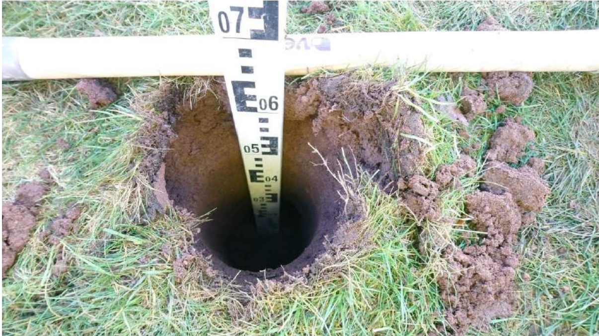
Photograph 13 Plot 12 showing 150mm of topsoil, 400mm of subsoil and 100mm granular break layer.
