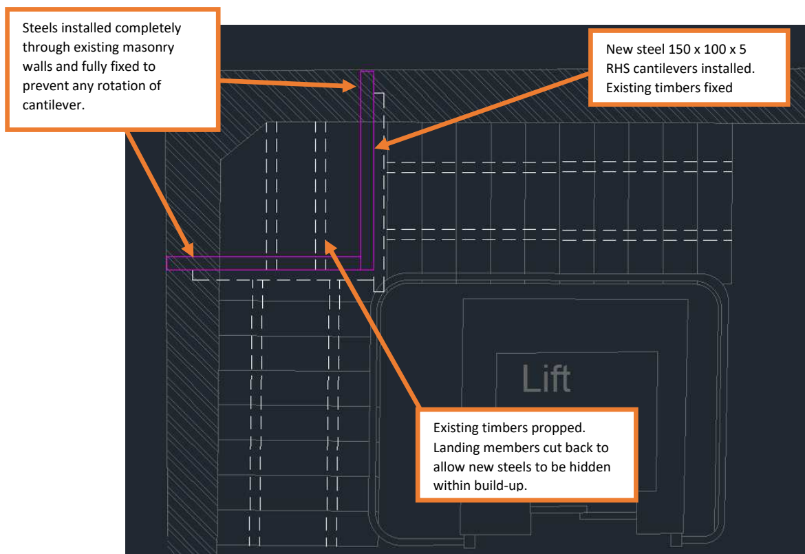
Image 7 – Proposed concealed remedial steel members.
