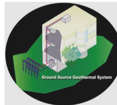
Ground Source Heat Pump Installation
