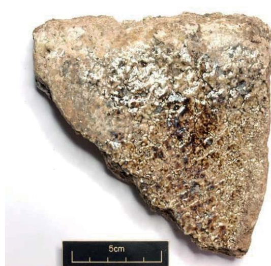
Plate 76: Refractory ceramic (lid/door?) from (143). Interior surface glazed by volatile alkalis from glass.
