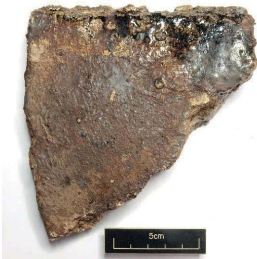
Plate 75: Refractory ceramic tile (lid/door?) from (047). Exterior surface glazed by coal ash/fumes.
