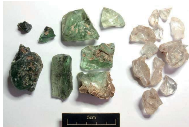
Plate 64: Glassworking waste from (140). Some examples are effectively colourless but most have a discernible green colour. The darker green examples sometimes show some contamination by clinker and/or partially burnt coal
