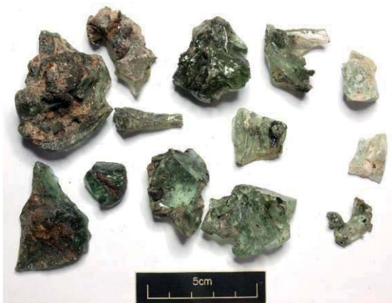
Plate 63: Glassworking waste from (047). A few examples are effectively colourless but most have a discernible green colour. The darker green examples usually show some contamination by clinker and/or partially burnt coal
