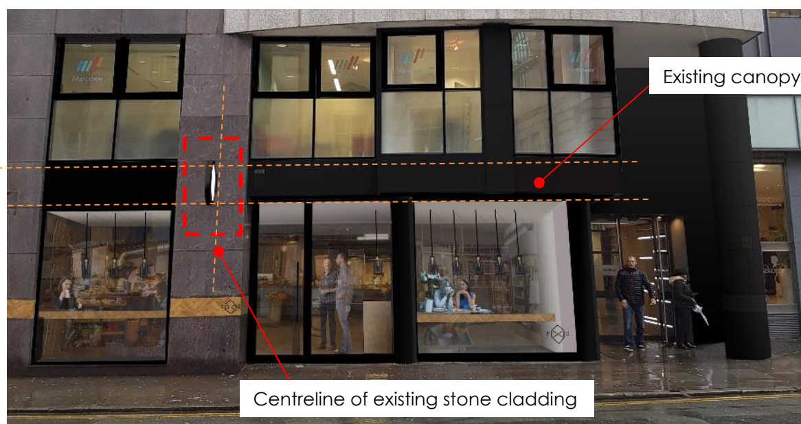
PROPOSED SHOPFRONT+SIGN_showing setting out/lining through with existing features
