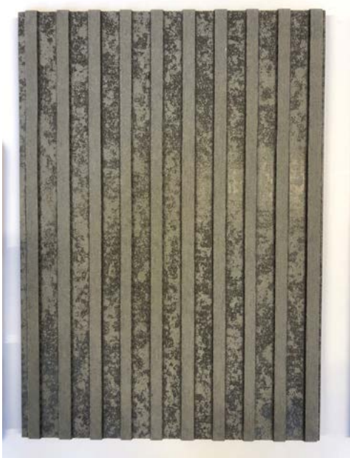
(A) Equitone Linea Fibre Cement Rainscreen Cladding 10mm flat panel, Textured, Marley Colour: Mid Grey, (Pebble) Secret fixing on Ground and First floors, exposed fixings above with austenitic stainless steel fasteners.
