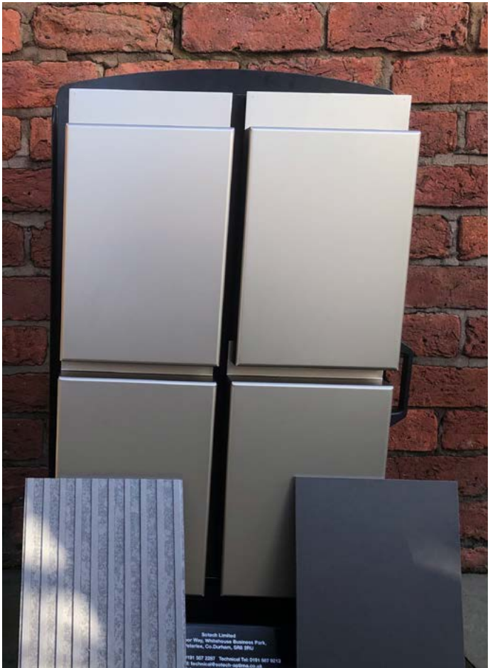
(C) Anodised Aluminium Rainscreen Cladding - Optima FC Secret Fix (J) Pale Gold Canopy Flashing (K) Pale gold Anodised Aluminium Extruded Fins Colour: Anodised Pale Umber, Rainscreen cladding system, drained and back ventilated, 3mm anodised aluminium panel of pale umber finish colour, vertical aluminium extruded fins adjoining aluminium cladding PPC colour and finish to match adjacent cladding, Canopy flashing in aluminium colour and finish to match aluminium rainscreen.
