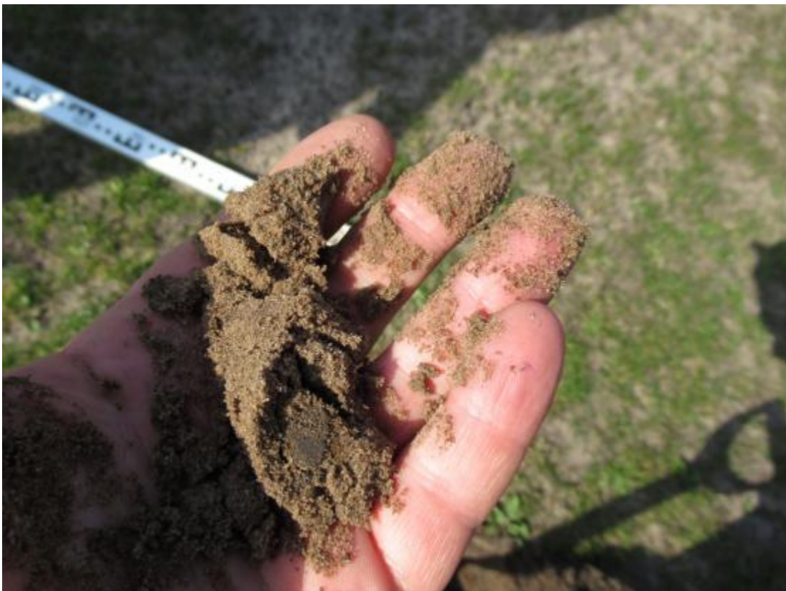
Sand layer at around 150mm depth is of a good quality medium-fine sand
