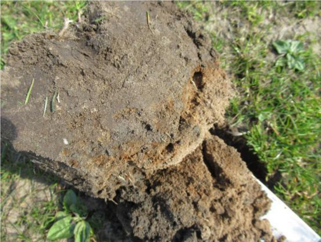
Very compact topsoil to 100mm depth, limited rooting, over sand layer
