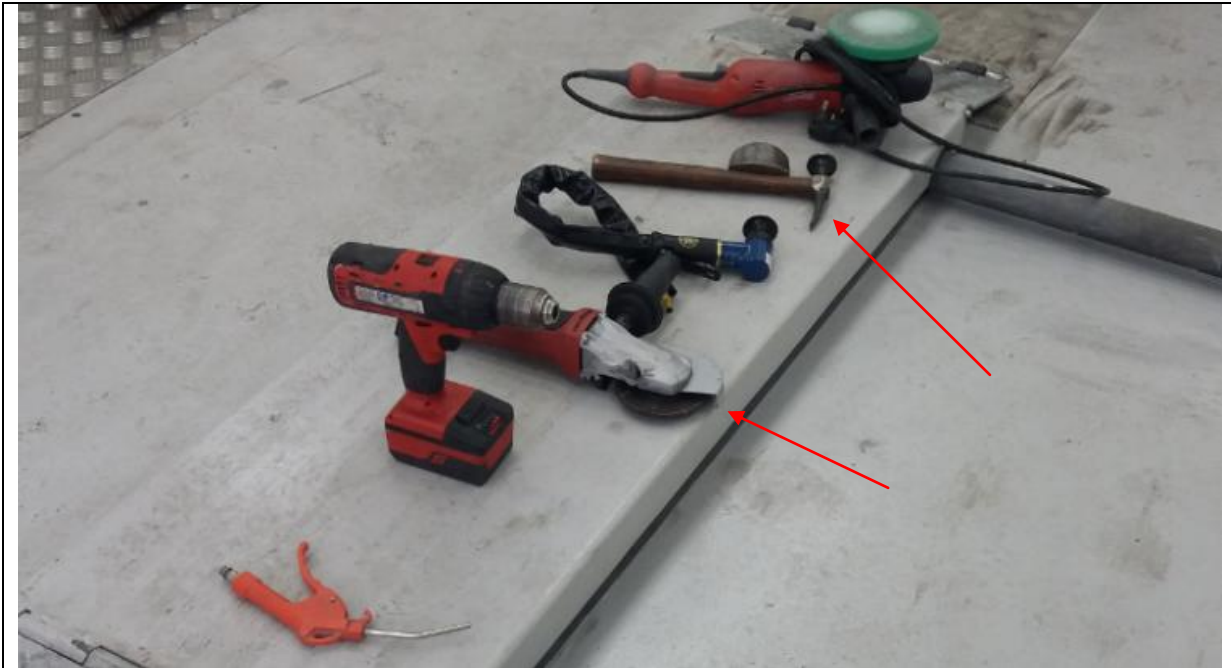
Above shows the types of equipment used on the vehicle repair processes: The Grinder and Hammer being noisiest.
