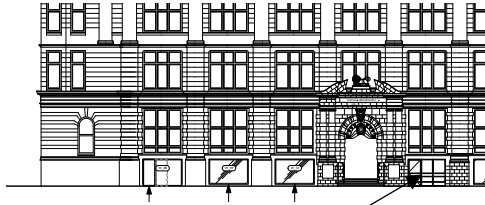
Existing entrance to disabled lift from Oxford Road affording full access to basement and lobby floors
