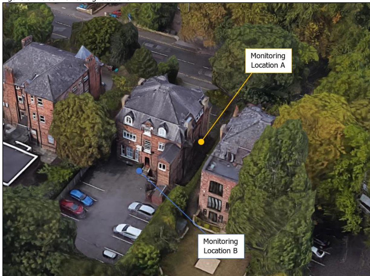
Figure 3: Noise monitoring locations
