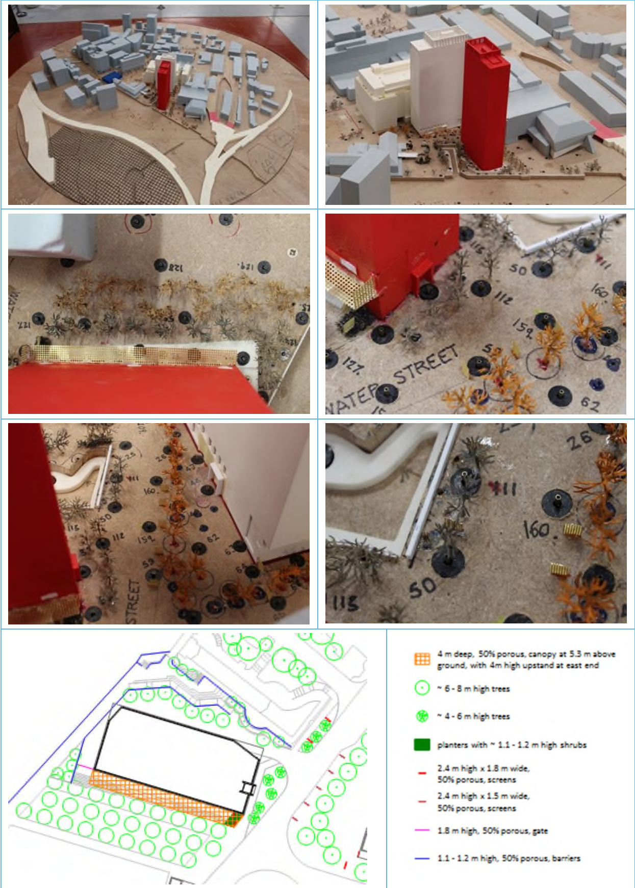
Figure A11.2c - Wind Tunnel Model, Close ups of Additional Mitigation with Interim Surrounds
