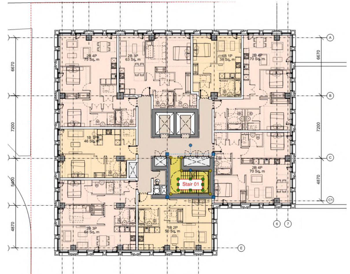
Figure 8 Level 9-16 general arrangement
