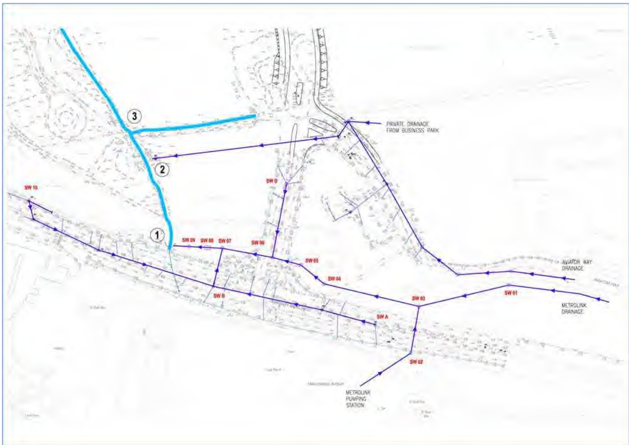
Figure 1.3 – Existing Drainage around the Aviator Way Junction
