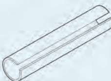
VT007 Slitted Carrier Pipe ● I.D. 100mm, length 6m, standard slit 30mm full length (10, 20 or 50mm slit also available).
