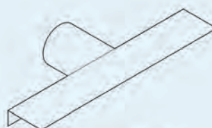
VT012 Gas Vent Outlet ○ VT011/25 (Width 915mm, connector length 190mm) to fit Gasflow 25 and VT006 100mm I.D pipe.
