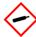
Gas Under Pressure
