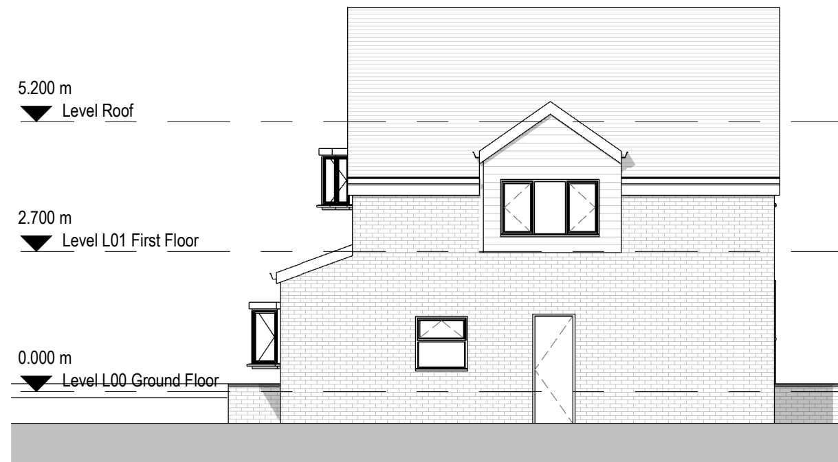
4 Existing East Elevation 1 : 100
