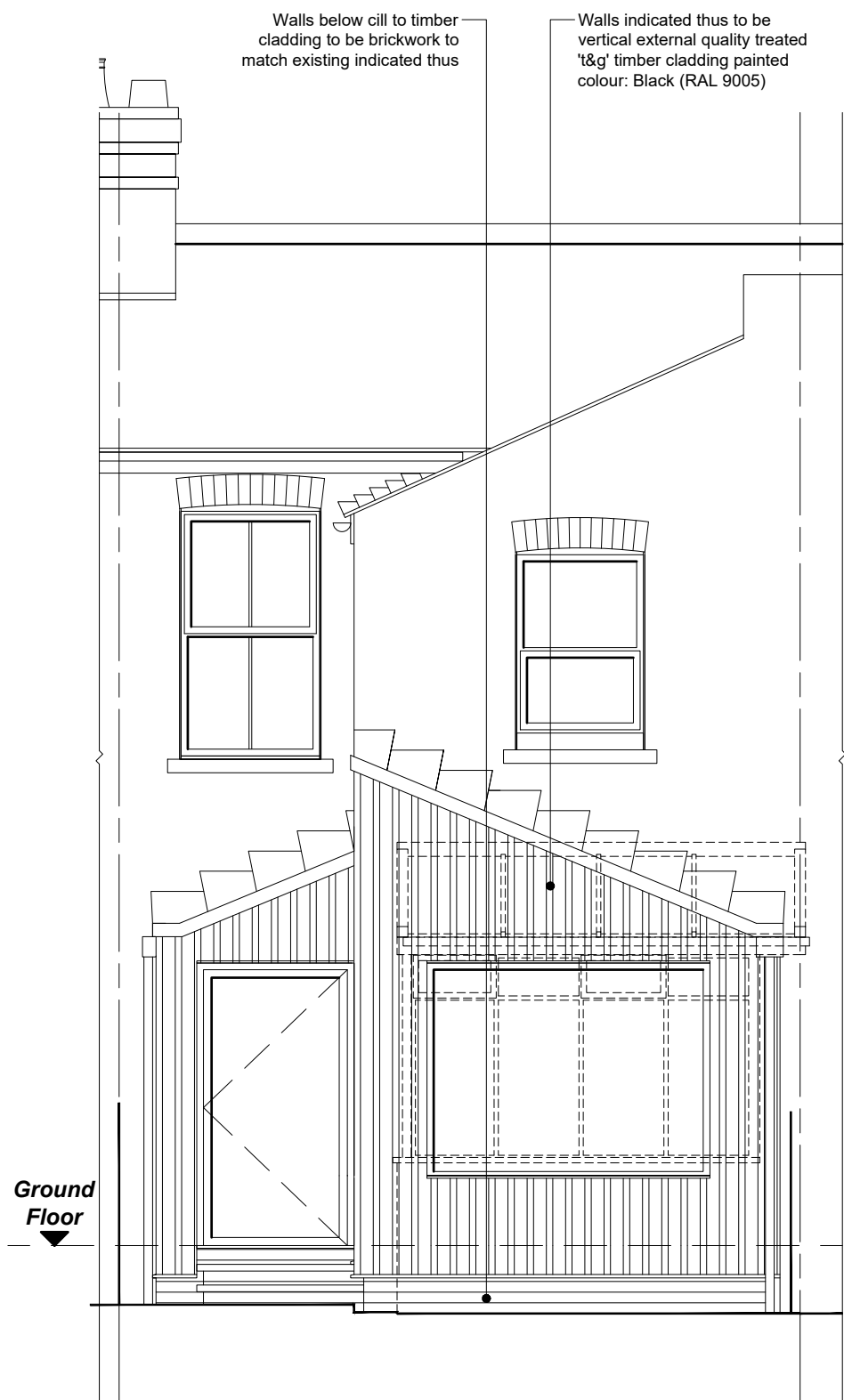
PROPOSED REAR (NORTH EASTERN) ELEVATION
