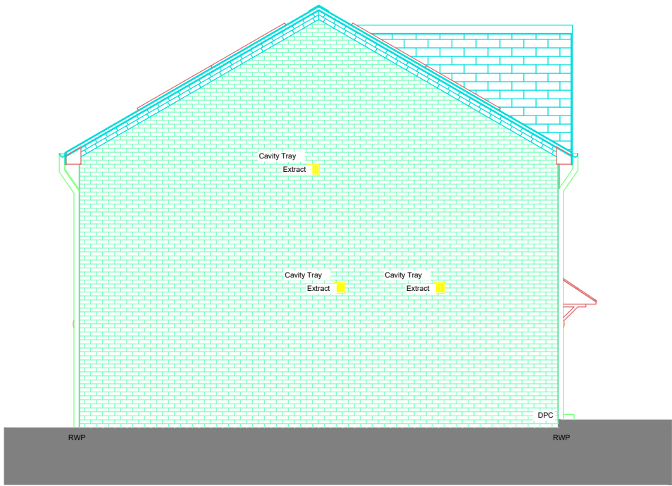
Existing Left Side Elevation
