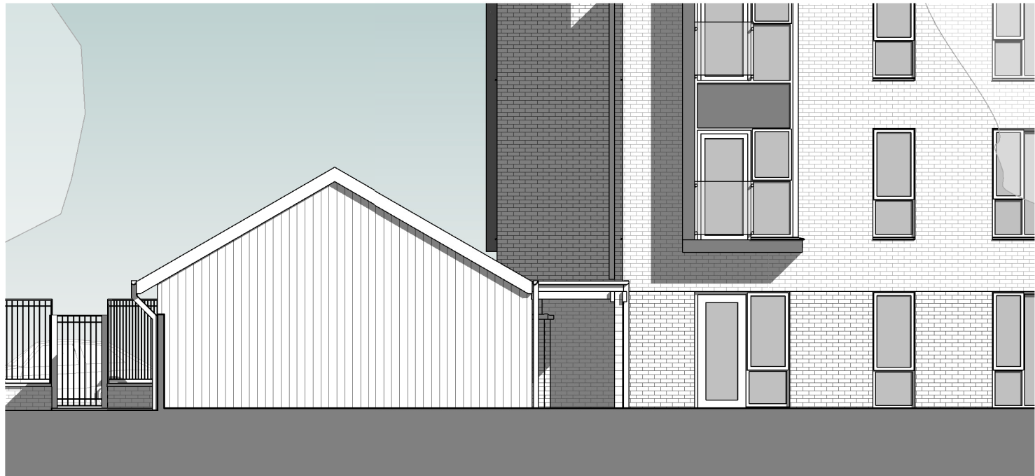
4 Residential Waste Container & Cycle Store - West Elevation 1 : 100
